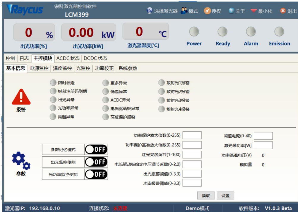
Figure 16 Main control module status information interface
