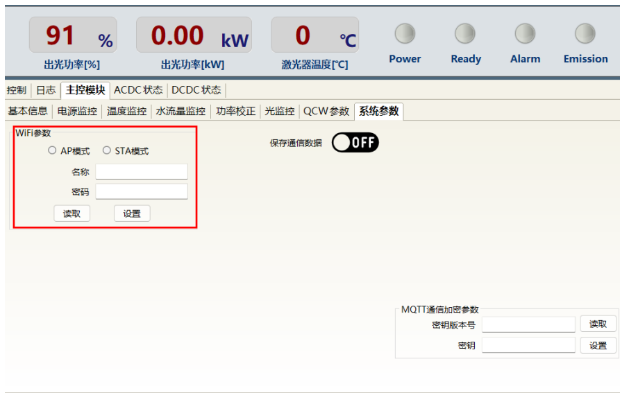
Figure 18 Main control module system parameter interface
