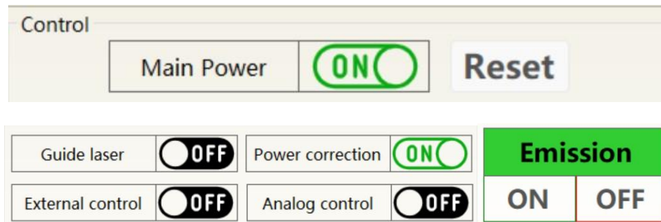
Figure 43 Display area for laser power on, mode selection, and light output control
