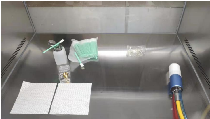
Figure 17: Output optical cable placed in a clean workbench with ventilation turned on
